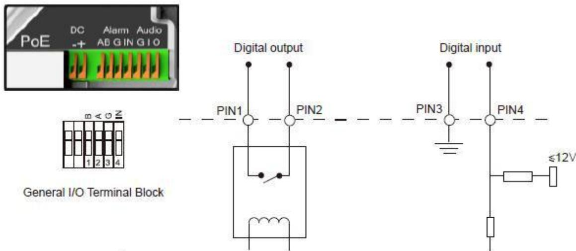
PIN1: Alarm Output NC/NO 24V DC 1A
