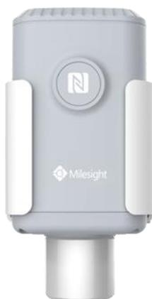
EM500-CO<sub>2</sub> is designed for measuring CO<sub>2</sub>, temperature, humidity and barometric pressure in harsh environments and transmitting data using LoRaWAN<sup>®</sup> technology. With this low power consumption technology, EM500-CO<sub>2</sub> can work up to 10 years with 19000 mAh battery. Combining with Milesight LoRaWAN<sup>®</sup> gateway and Milesight IoT Cloud solution, users can manage all sensor data remotely and visually.
